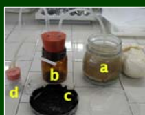
Figure 2. Collecting springtails: (a) laboratory culture, (b) insect aspirator, (c) Petri dish, (d) weighing bottle with aspirator
