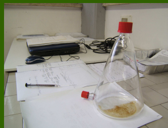
Figure 4. Flask with defatted meal and water used to evaluate the allyl-isothiocyanate release over time by the headspace analysis
