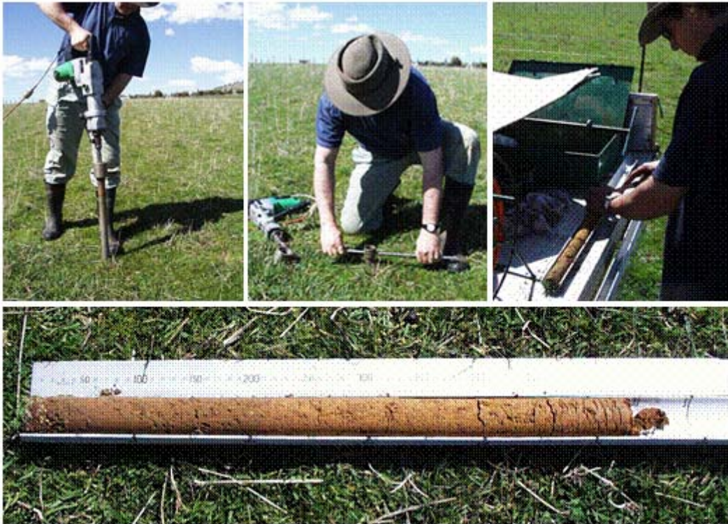
Figure 1. Soil core collection and examination during an initial survey of soil profiles across a paddock.
